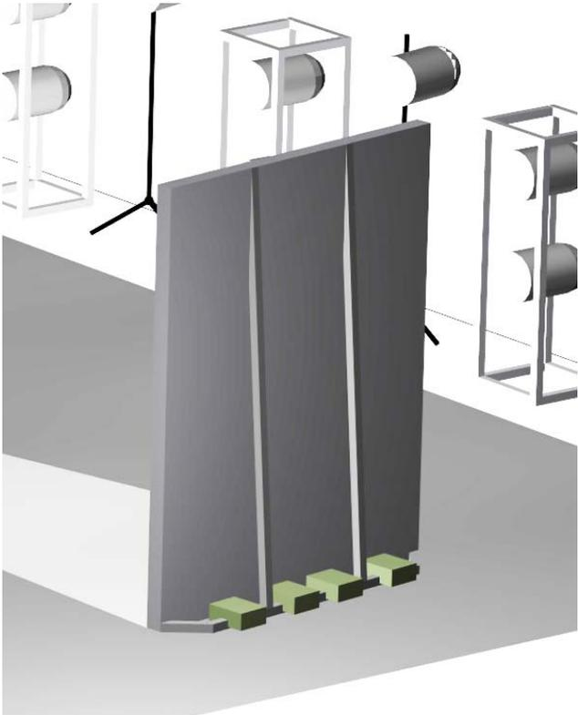
The weights, in green, can be metal blocks, sandbags or anything that is heavy enough to stabilize the frame, holding it firmly to the ground.
